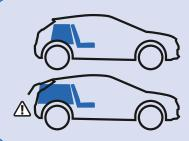
Variocage is adjustable in length. The slope of the front, back and sides are angled so it can easily fit in a typical cargo area while also providing maximum room for your dog. If you have a cargo door with a steep angle, it may not close properly with the crate fully extended. Consider the final adjusted length of the cage to be sure it will offer enough space for your dog. For shorter cargo areas, a Variocage Double with the centerdivider removed will offer more room for 1 or 2 dogs.
