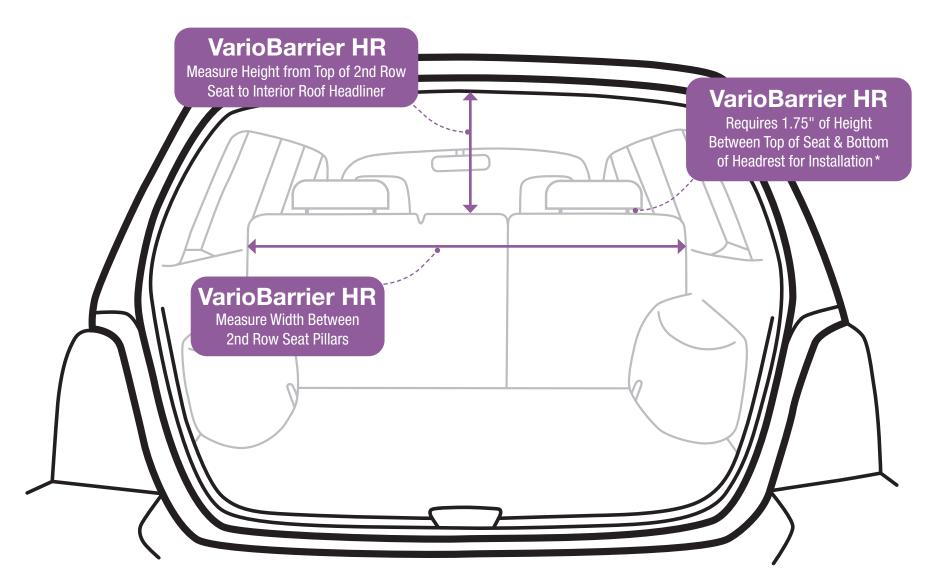
\*The VarioBarrier requires a Straight Headrest Post and 1.75" between the Top of the Seat and the Bottom of the Head Rest for Installation. VarioBarrier will not work with curved or angled Headrest Posts. In this case, please use our VarioBarrier instead of the VarioBarrier HR.
